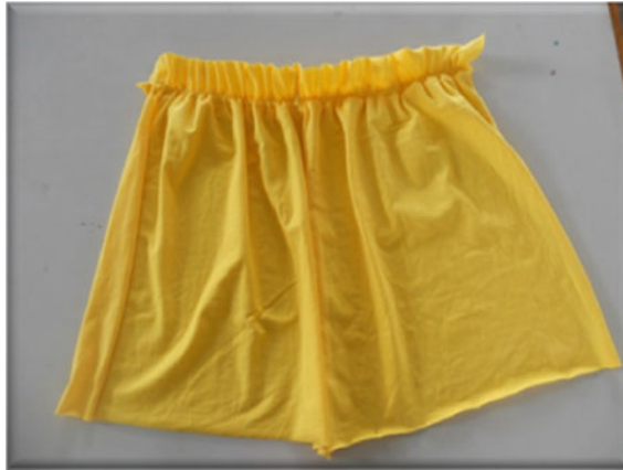
Fig. 21 Preparation of gathers and attachment of waistband with skirt
