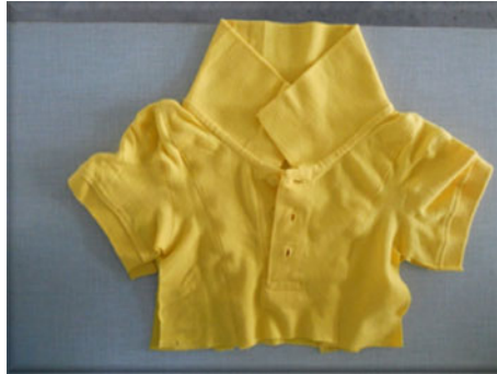
Fig. 39 Attach the neck portion along with the chest and sleeve panels
