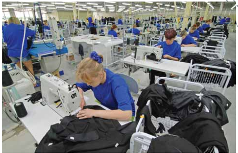
A machinist in a factory often works on only one part of a garment, which then moves on for the next stage in the production process.
