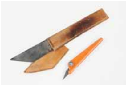
A Utility Knife or Craft Knife is used to cut leather. A Leather Shear can also be used to cut leather, suede and plastics.
