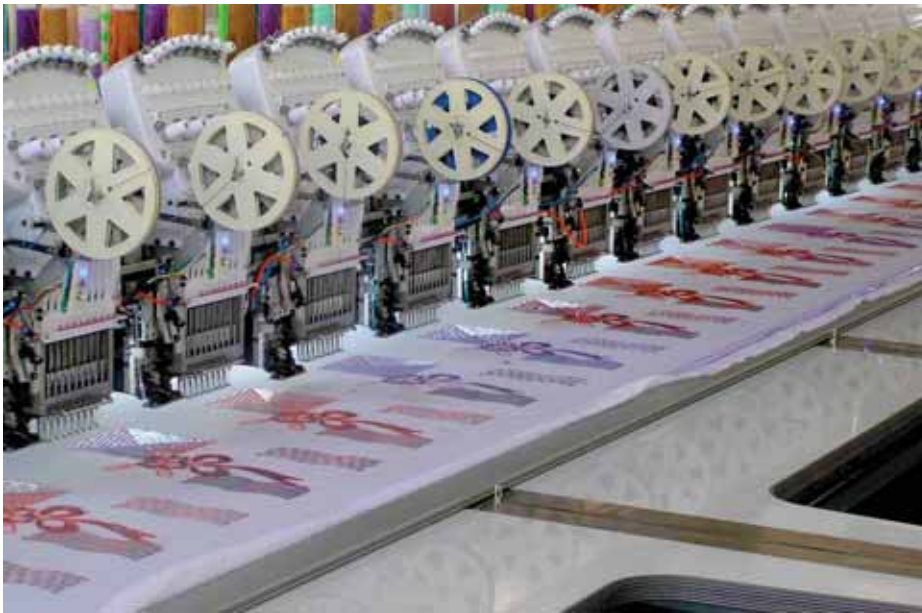
An industrial embroidery machine can reproduce many copies of the same design in different colourways.
