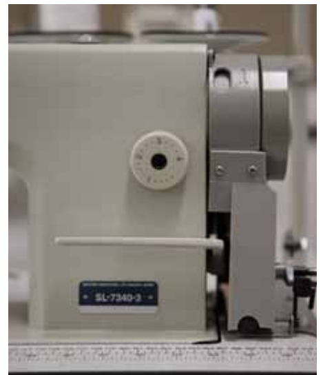
A stitch regulator on an industrial flatbed sewing machine. On this machine the stitch length can vary from 0–4mm.
