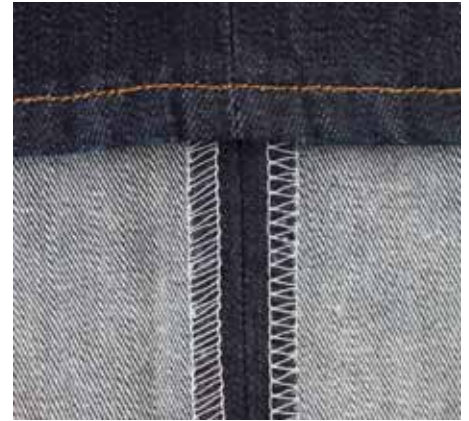
The side and inside leg seams may be stitched with a plain seam pressed open or to one side, towards the back, with seam allowances overlapped together.
