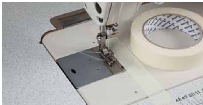
Alternatively, or if the sewing machine is not equipped with a sewing guide, place a strip of masking tape onto the throat plate as a guide for the sewing line.
