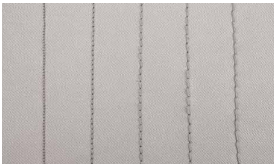
From left to right: Stitching lines with a stitch length of 1mm, 2mm, 3mm, 4mm and 5mm.
