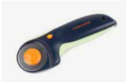
A Rotary Cutter has a circular blade that rotates. It comes in different sizes and blade shapes. The rotary cutter is best used when cutting several layers of material at the same time. This tool is recommended when looking for a straight line with angled rather than curved corners, such as patchwork pieces. It can also be used for cutting leather and non-woven materials such as PVC. Always use a cutting mat underneath the material otherwise the cutting lines will mark the surface beneath.
