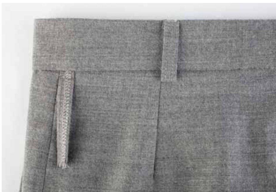
A belt loop attached to the waistline before the waistband is stitched on. Once the waistband is attached, the belt loop is secured with enough ease to allow for a belt.
