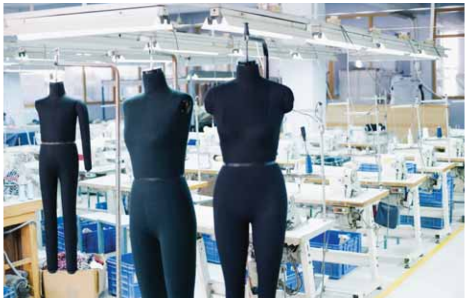
Dummies are used during the initial construction of made-to-measure garments.
