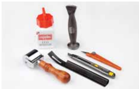
Front row, left to right: roller to flatten seams, skiver knife to reduce bulk, Stanley knife and craft knife for cutting. Back row, left: adhesive to glue seams and hem allowances down; right, hammer device to flatten seams.
