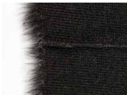
Fabric fur seam with zigzag stitch.
