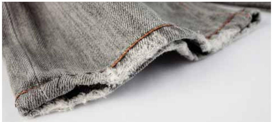
Jeans usually have a double-turned hemline, topstitched down with a topstitching thread. A distressed look is typical in denimwear, especially at the hem edge.
