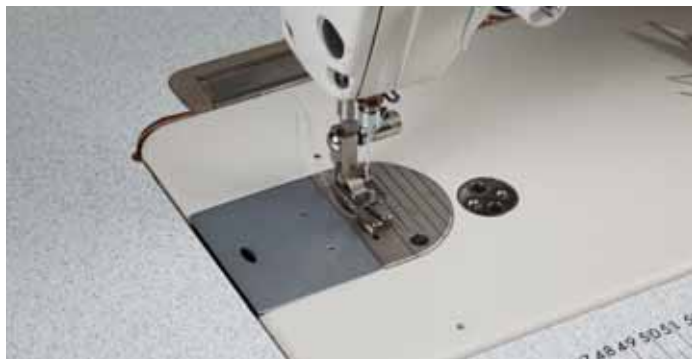
A flatbed machine with sewing guidelines engraved onto the throat plate.
