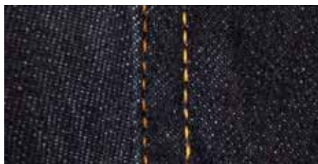
Flat fell seam topstitched with two different colours of thread to create a subtle design feature.
