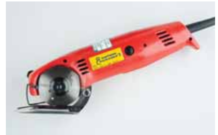
A Rotary Cutter has a circular blade that rotates. It comes in different sizes and blade shapes. The rotary cutter is best used when cutting several layers of material at the same time. This tool is recommended when looking for a straight line with angled rather than curved corners, such as patchwork pieces. It can also be used for cutting leather and non-woven materials such as PVC. Always use a cutting mat underneath the material otherwise the cutting lines will mark the surface beneath.
