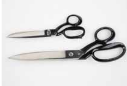
Shears come in two sizes, medium and heavy; the choice of size depends on the weight of the fabric. Bent-handled shears allow the blade to lie flat on the cutting surface; they are more comfortable to use and allow better control.
