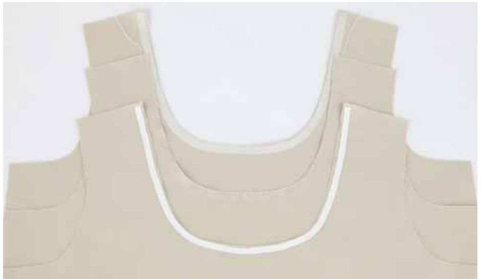
From top to bottom: Iron-on, stay-stitched and taped necklines.
