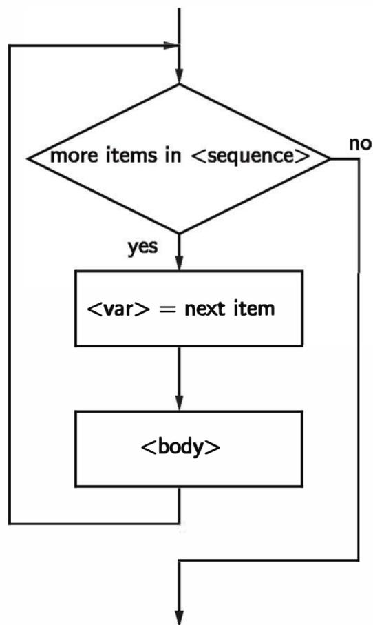
Figure 2.3: Flowchart of a `for` loop
