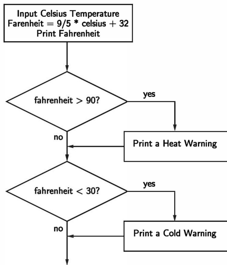
Figure 7.1: Flowchart of temperature conversion program with warnings
