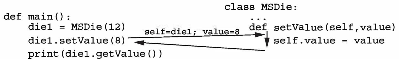
Figure 10.2: Flow of control in call: `die1.setValue(8)`
