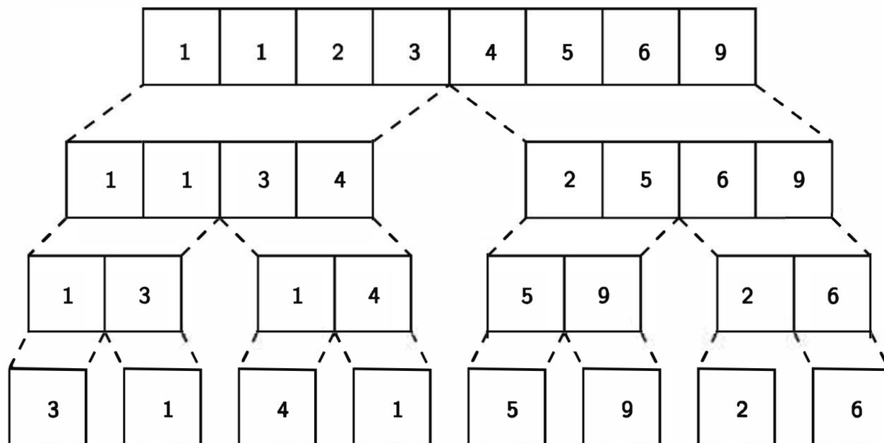
Figure 13.3: Merges required to sort [3, 1, 4, 1, 5, 9, 2, 6]
