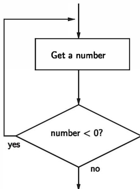
Figure 8.2: Flowchart of a post-test loop
