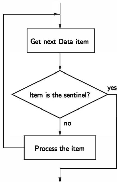
Figure 8.3: Loop-and-a-half implementation of sentinel loop pattern
