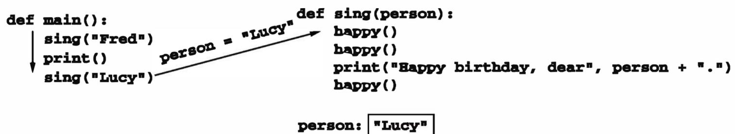
Figure 6.4: Snapshot of second call to sing
