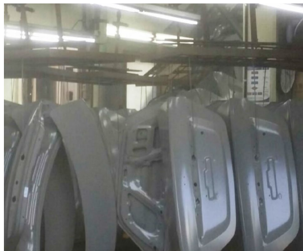
(a) Large components attached to hangers
