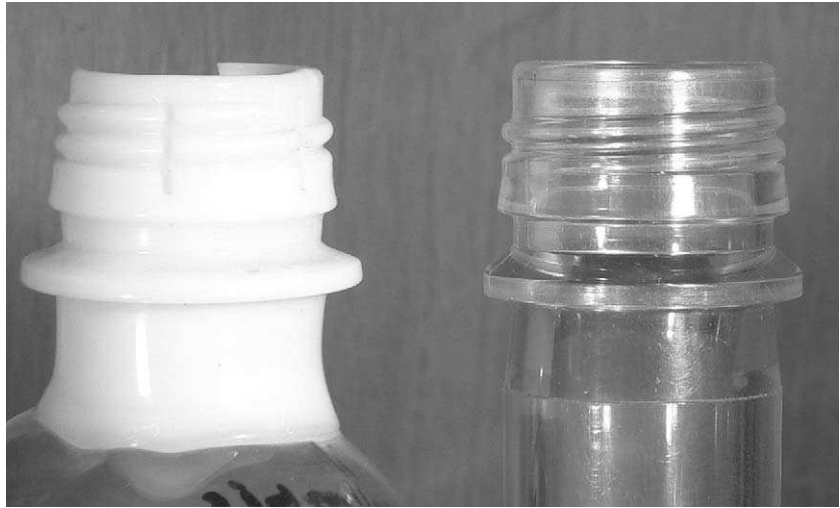
Figure 1.17 Details of the neck region of an injection-blow moulded PET bottle. The bottle on the left has been heat treated at 120 °C, while the neck of a preform is shown on the right.
