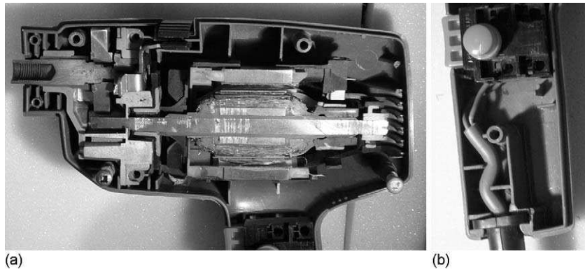
Figure 13.18 A sectioned electric drill, showing internal ribs that locate the: a) the motor and gearbox, b) the mains cable
