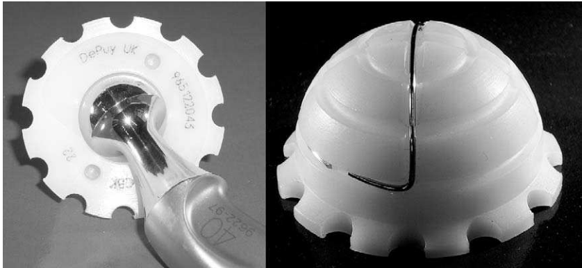
Figure 15.13 Charnley acetabular cup design showing grooves on exterior for bone cement, and the stainless-steel wire for wear assessment by X-ray.
