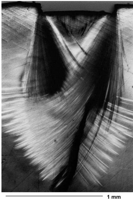
Figure 8.1 Pattern of shear bends in a block of polystyrene, under a strip indenter.
