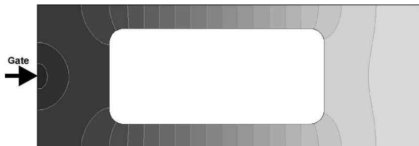
Figure 5.26 Isobars for two-dimensional isothermal flow into a mould, computed using a thermal heat flow analogy.
