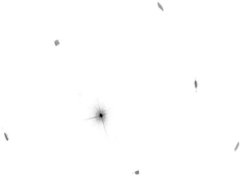
Figure 1.10 Diffraction pattern from a laser pointer, when shown on the track near the end of a music CD; the direct reflection has the cross pattern.
