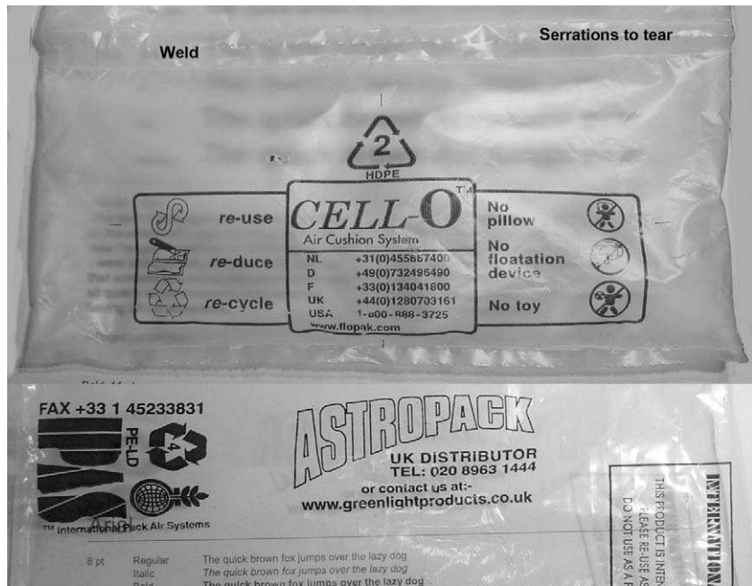
Figure 1.11 LDPE and HDPE macro-bubbles (deflated) on top of a test page with a range of font sizes.
