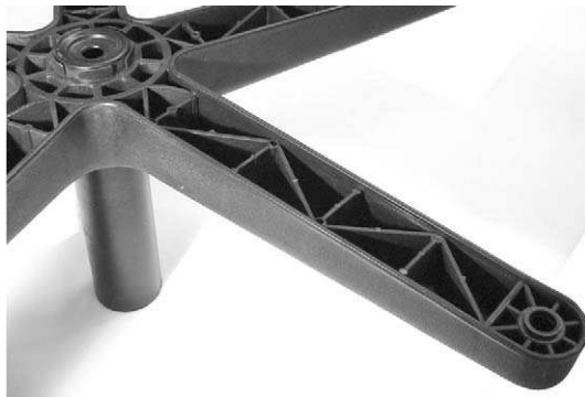
Figure 13.15 Diagonal rib pattern, on the underside of office chair legs, that provides bending and torsional stiffness.
