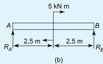
$$[R_A = -1 \text{ kN}, R_B = 1 \text{ kN}]$$
