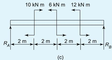
$$[R_A = 1 \text{ kN}, R_B = -1 \text{ kN}]$$
