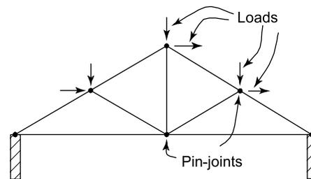
Figure 6.1 Pin-jointed truss
