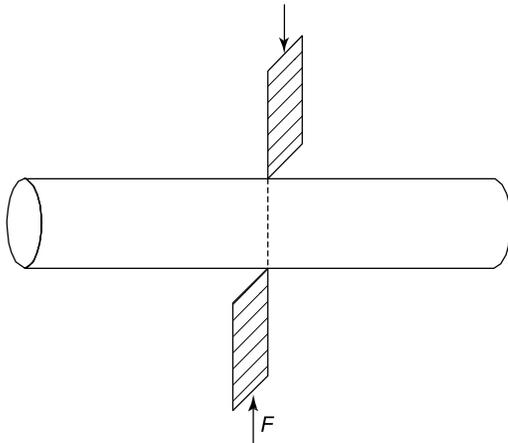
Figure 7.3 Shearing action
