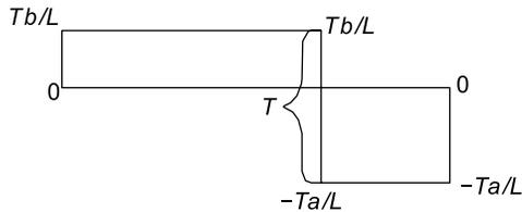
Figure 11.6 Torque diagram
