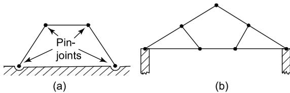
**Figure 6.4** Mechanisms
