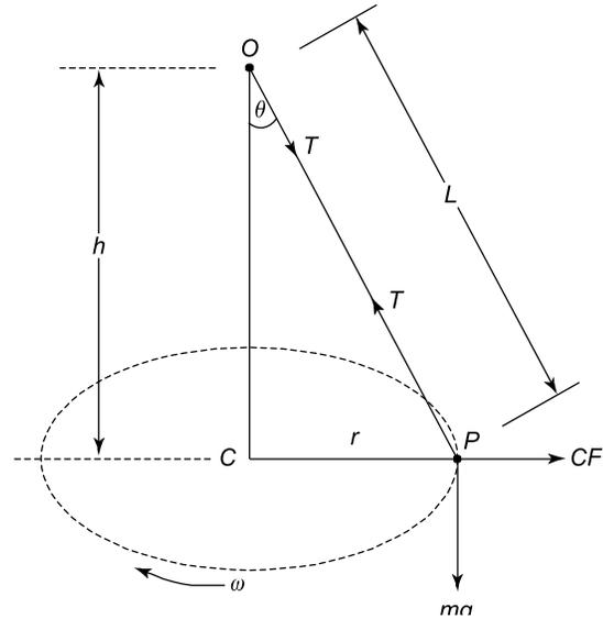
Figure 17.5 Conical pendulum
