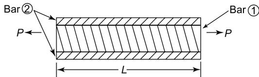
Figure 2.14 Compound bar under axial tension
