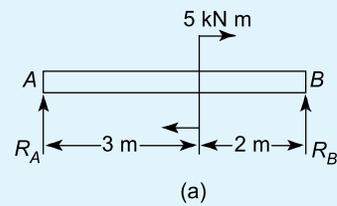
$$[R_A = -1 \text{ kN}, R_B = 1 \text{ kN}]$$
