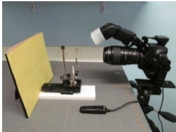
Image 85 - Basic focus stacking setup
