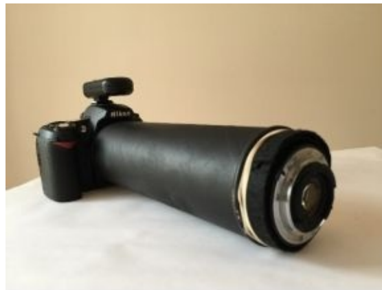
Image 72 - Final DIY Extension Tube Wth Reverse Lens
