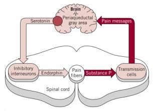
**Figure 11-3** Illustration of the chain of activity involved in SPA. Stimulation to the periaqueductal gray area of the brain starts a sequence of electrochemical reactions, eventually leading to inhibition (shown by shaded arrows) of the pain fibers' release of substance P, thereby reducing pain messages from the transmission cells to the brain.
