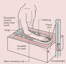
**Figure 11-1** Apparatus for the cold-pressor procedure.
