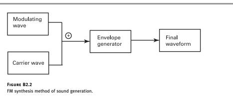
modulating wave. Many FM chips used four or six oscillators for each sound, or instrument. An oscillator could also be fed back on itself, modulating its original sound.
