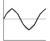
FIGURE B2.3 Bit depth, showing a 4-bit sample.
