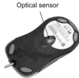
Fig. 4.3 The lower portion of the optical mouse
