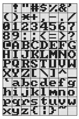
These are the characters corresponding to ASCII codes 20h through 7Fh. (No visible characters are associated with ASCII codes 00h through 1Fh.)
