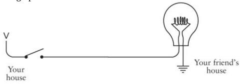
The V stands for *voltage*, but it could also stand for *vacuum*. Think of the V as an electron vacuum and think of the ground as an ocean of electrons. The electron vacuum pulls the electrons from the earth through the circuit, doing work along the way (such as lighting a lightbulb).
