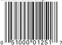
We're tempted to try to visually interpret the UPC in terms of thin bars and black bars, narrow gaps and wide gaps, and indeed, that's one way to look at it. The black bars in the UPC can have four different widths, with the thicker bars being two, three, and four times the width of the thinnest bar. Similarly, the wider gaps between the bars are two, three, and four times the width of the thinnest gap.
