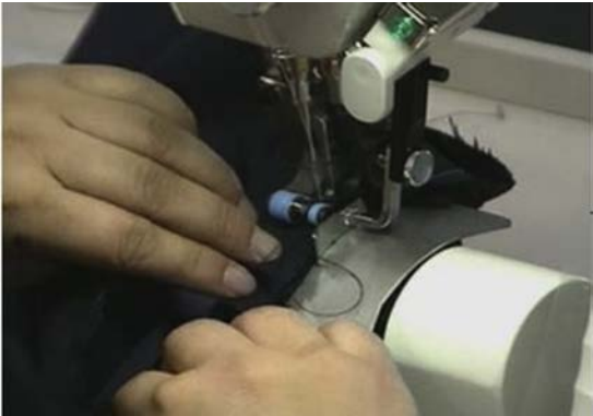
Figure 13.31 Workplace for attaching sleeves.
