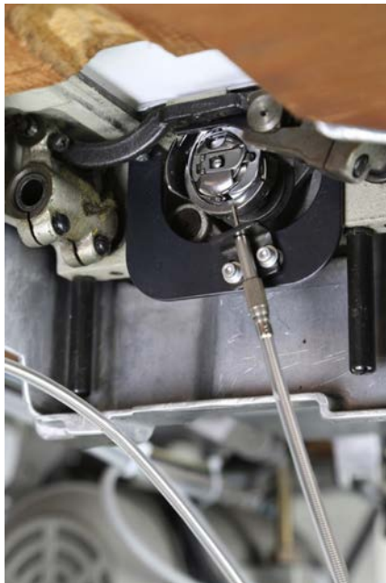
Figure 9.25 Automatic bobbin checker by Kinoshita.
