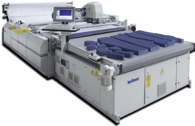
Figure 2.10 Automatic cutter PROCUT from Bullmer.
