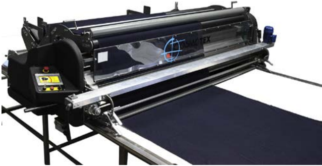
Figure 6.1 The automatic spreading machine, Apollo Smart 300 by Cosmotex.
