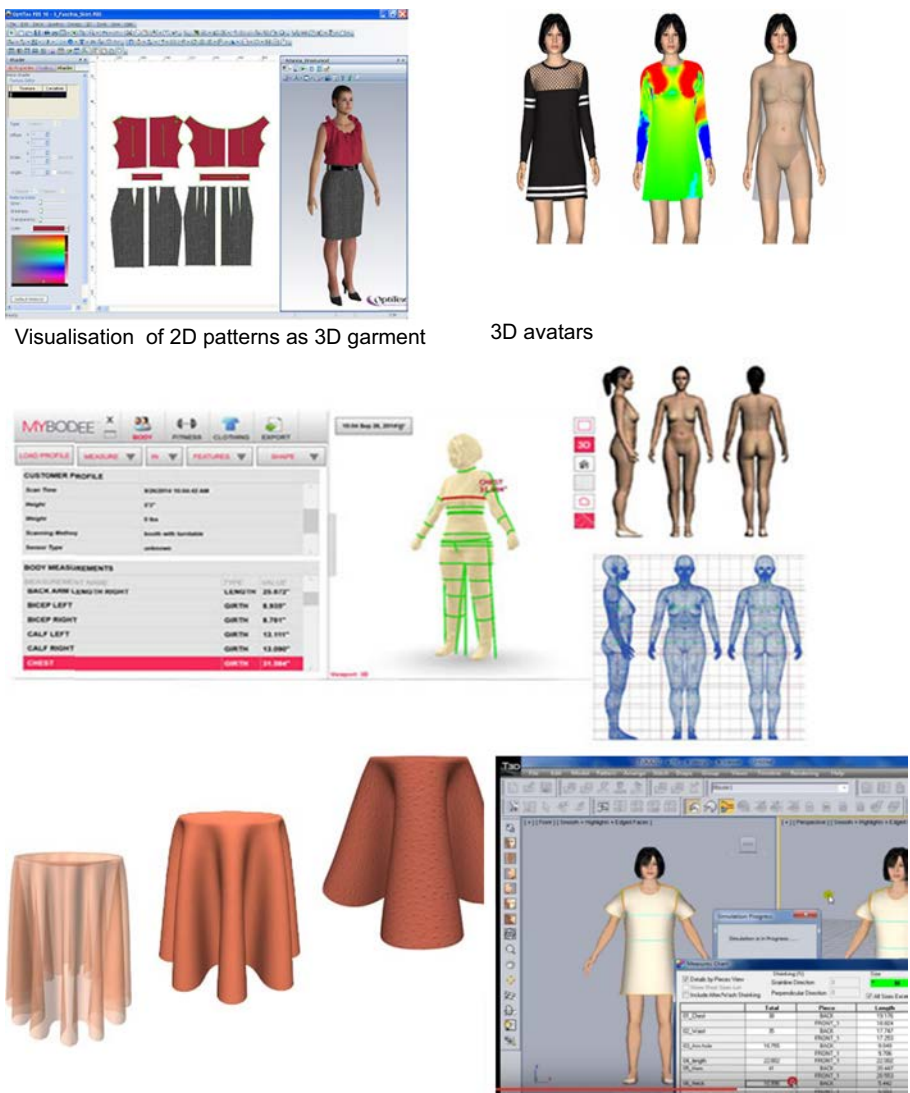
Figure 11.17 Creation of 3D avatars and visualization of garments’s drape and fit in dynamic and static postures.
