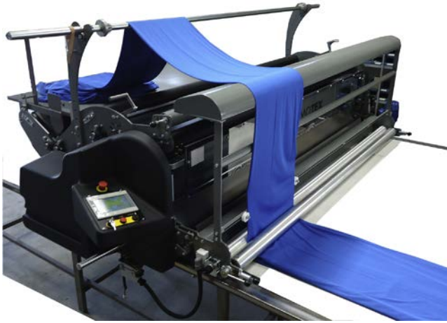
Figure 6.3 The automatic spreading machine Apolo Smart 300 by Cosmotex equipped with several special devices to lay tubular fabrics.
