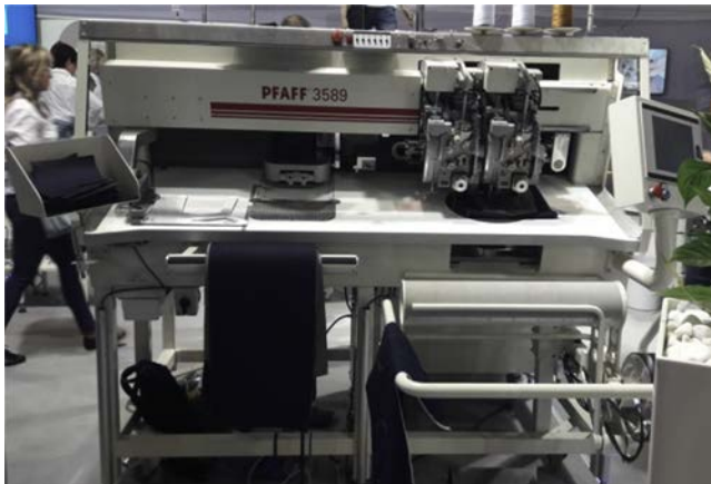
Figure 2.17 PFAFF industrial automatic sewing system.
