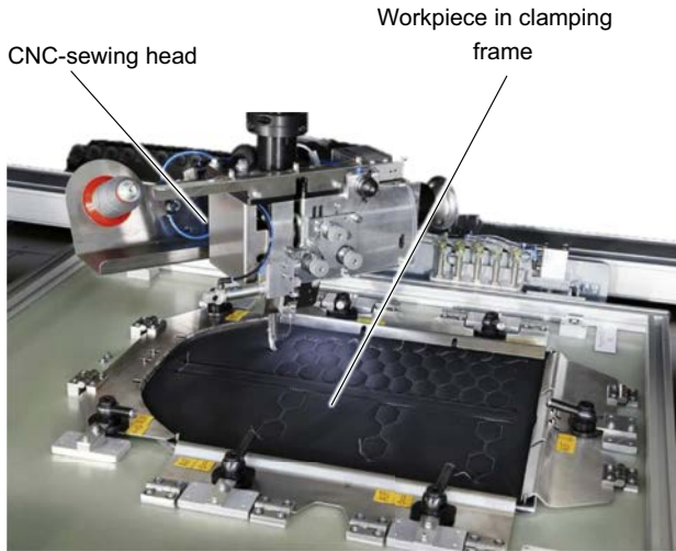
Figure 8.5 Computer numerical control-sewing machine for ornamental seams for car seats.
