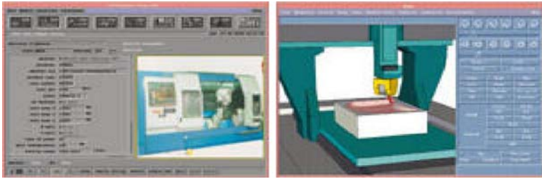
Figure 11.1 Computer-aided design/computer-aided manufacturing application in mechanical field—library of machine tools and graphical simulation.
