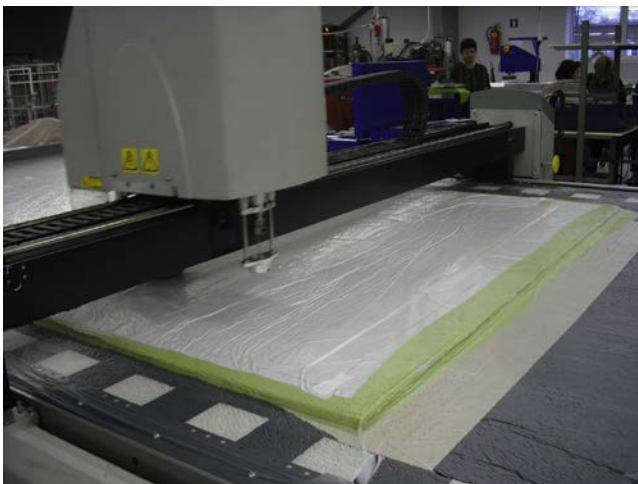
Figure 6.9 The fabric spread covered with polyethylene film during the cutting process.
