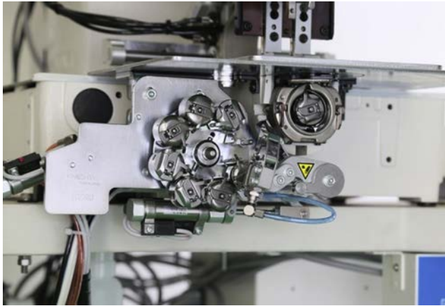
Figure 9.26 Automatic bobbin changer by Kinoshita.
