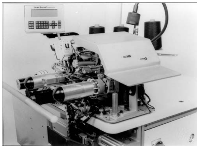
Figure 9.30 Rib attaching at bottom hem of sweatshirts (Union Special).
