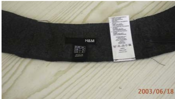
Figure 13.16 Case study: attaching labels to the lining of the waistband.
