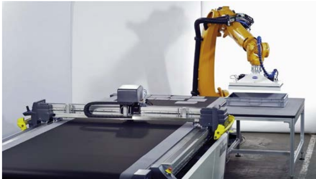
Figure 2.16 Bullmer and KUKA robots with vacuum gripper manipulate pattern pieces.
