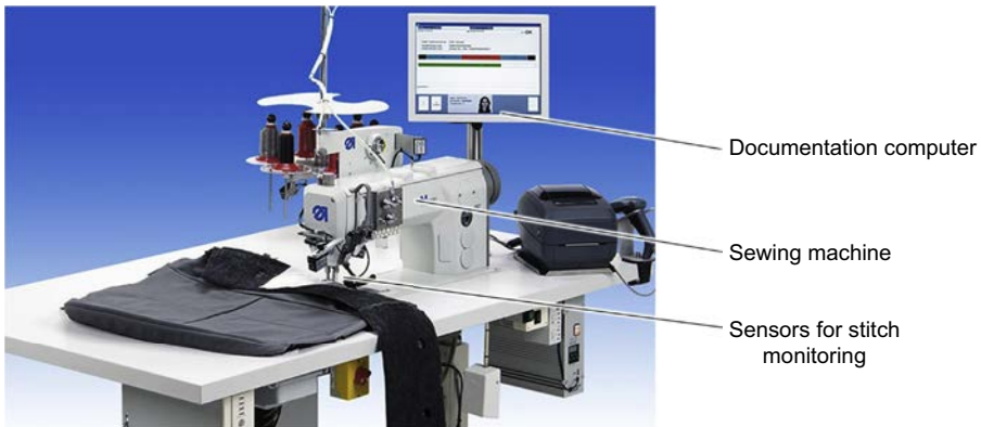
Figure 14.11 Dürkopp Adler seam documentation system for creation of airbag seam.
