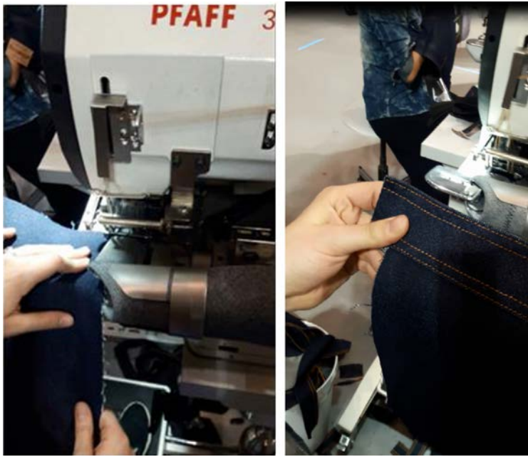
Figure 2.18 PFAFF industrial automatic sewing machine for waist belt.
