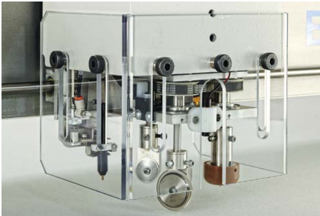
Figure 6.5 The cutting head with tools of a single-low ply cutter by Eastman.
