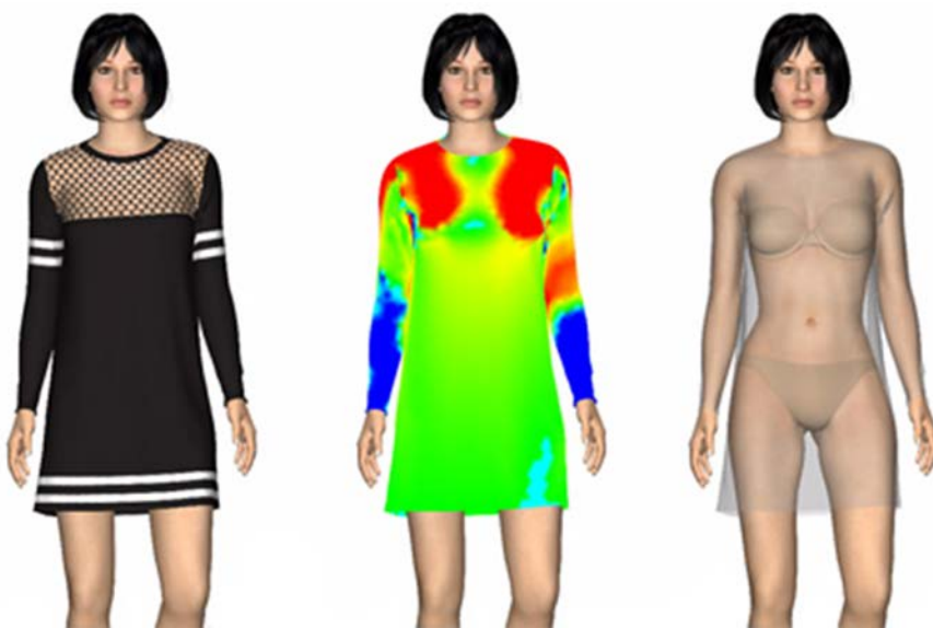
Figure 10.9 Example of a virtual fit ( www.tukatech.com ). Left side: complete view; Middle: visualization of tightness of fit; Right side: transparent view.
