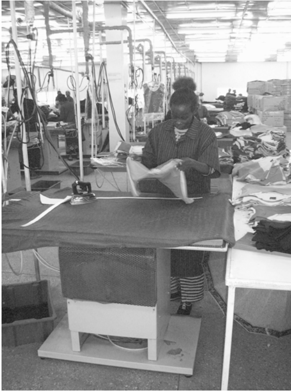
12.1 A basic industrial ironing station; the last stage of a making-up line. (Courtesy of Sun Flag Ltd, Arusha, Tanzania.)
