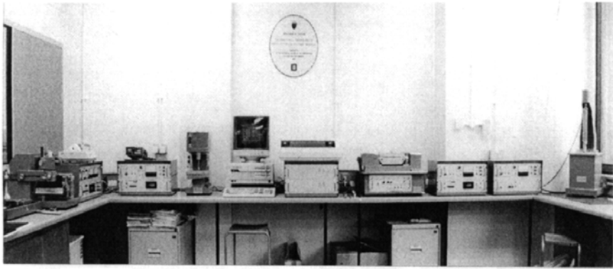
1. Surface tester 2. Compression tester 3. Data system 4. Shear tensile tester 5. Pure bending tester
