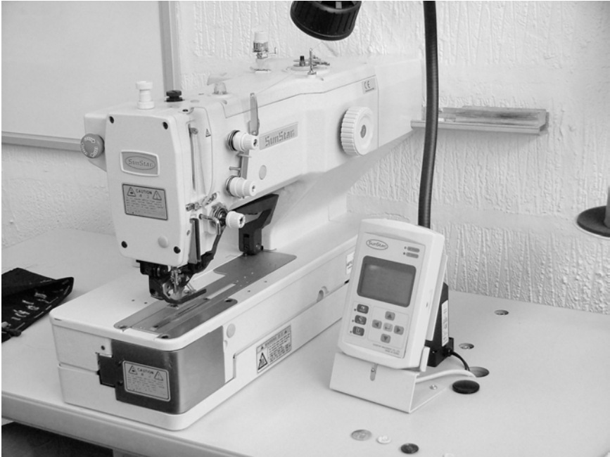
10.13 Electronic buttonholing machine.
