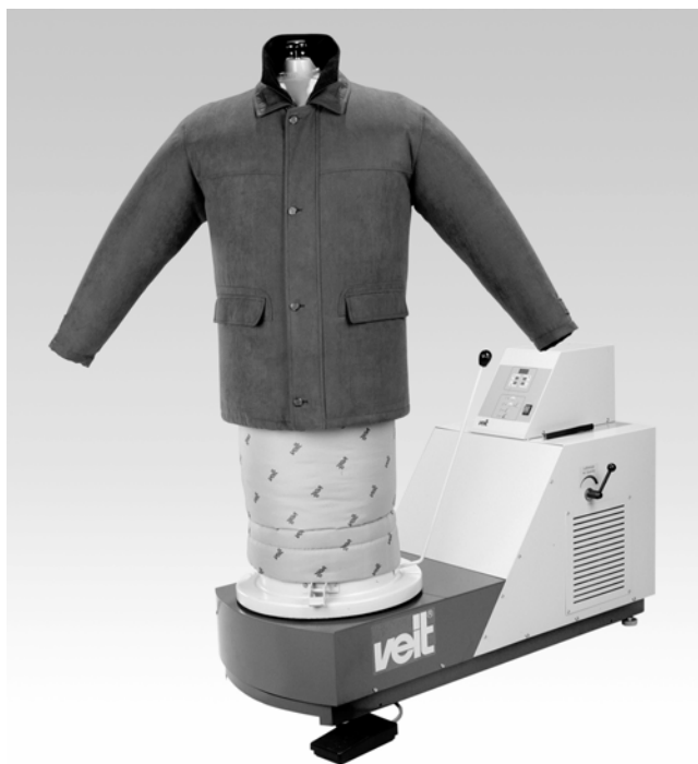
12.6 Blouse dolly finisher. (Courtesy of Veit Kannegiesser GmbH, Vlotho, Germany.)
